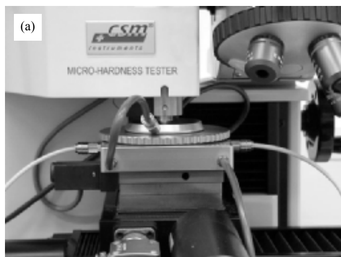
Figure 1 : Heating/cooling stage mounted on the Micro Hardness Tester to give an effective sample temperature range of -35°C - 450°C. The sample is mounted in the centre of the stage and is accessed by the indenter through a small aperture (a). Subsequent imaging is performed by displacing the stage under the integrated optical microscope.
